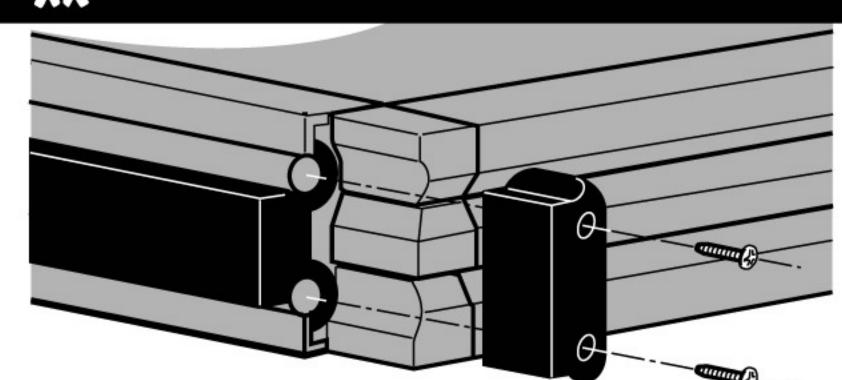
To remove foreign matter from panel hinges, remove one end cap and slide panels apart. Reassemble after cleaning.
